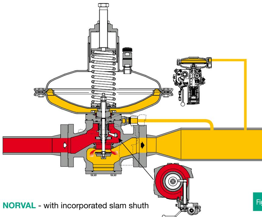
The slam shut valve can be set for pressure increase, **over pressure shut off (OPSO)** and/or for pressure drop, **under pressure shut off (UPS0)**.
