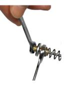
To re-assemble the slam-shut valve, follow the procedure described for disassembly in reverse order. Before reassembling the tightness elements (O-rings, membranes, etc.), it is necessary to check their integrity and, if necessary, replace them.
