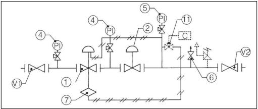
Figure 21: Monitor + Active Regulator Diagram (internal sensing line)
