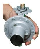
5. Unscrew the plug and the adjustment ring nuts. Then remove the calibration springs and the spring supports;
