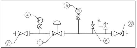
Figure 15: Dival diagram (internal sensing line)
