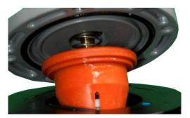
13. Separate the balancing assembly from the head by performing a shift in the gas flow direction so that the stem comes out from the towing coupling;
