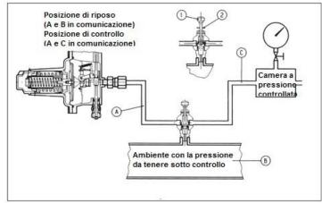
Figure 19: "Push" connection diagram
