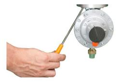
4. Remove the slam-shut device
