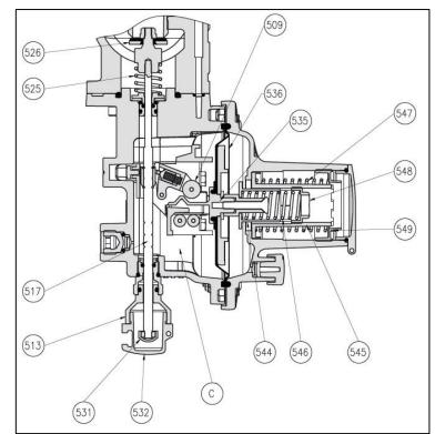
Figure 9: Slam-Shut Device LA
