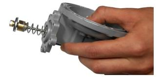
10. Unscrew the nut and remove the obturator
