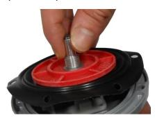
8. Remove the plug, unscrew the nut and ring nut
